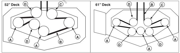
Figure 50. Mower PTO Belt Routing A. Spindle Pulley B. PTO Drive Belt C. Spring-loaded Idler Pulley D. Stationary Idler Pulley
